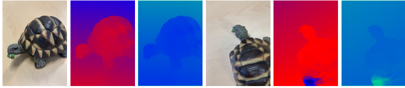
Fig. 5. Qualitative results with Apple iPhone XS. We show two examples of reference image and disparity map acquired with the iPhone XS, followed by estimated confidence map after few iterations of on-the-fly learning.
