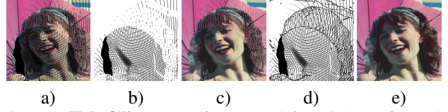
Figure 3. Hole filling strategies. From left to right: a) forward-warped image affected by stretching artefacts, b) holes mask \mathcal{H} c) inpainted image, d) collision-augmented holes mask \mathcal{H}' and e) improved inpainted image. Black pixels in \mathcal{H} and \mathcal{H}' are those to be inpainted.
